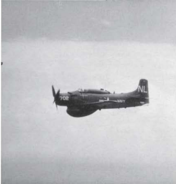
The Airborne Early Warning "Guppy" on station searched for low flying aircraft, submarines and other surface craft . . .
