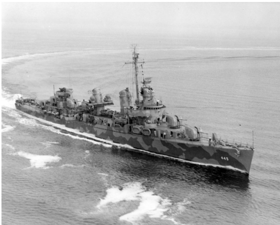
USS Fletcher (DD-445), the lead ship of the many destroyers of this class, in July 1942. This was the first five-gun destroyer to have all of her 5" (12.7 cm) guns in enclosed Mark 30 mountings. U.S. Naval Historical Center Photograph # 19-N-31243.
