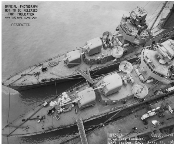
USS Blue (DD-387) outboard and USS Ralph Talbot (DD-390) inboard at the Mare Island Navy Yard, California on 11 April 1942. These ships were Bagley class (DD-386) destroyers that were armed with Mark 25 mountings on their bows. Note the Mark 33 Directors on top of their superstructures and that no radars had been installed at this time. Gun tubs in front of the bridges hold 20 mm Oerlikon autocannons . U.S. Naval Historical Center Photograph # 19-N-29229.
