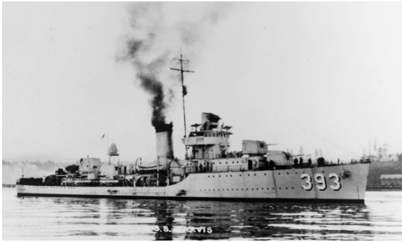
USS Jarvis (DD-393), a Bagley class (DD-386) destroyer, in 1937. This destroyer had two Mark 25 enclosed base ring mounts on the bow and two Mark 24 pedestal mounts on the stern. U.S. Naval Historical Center Photograph # 67842.
