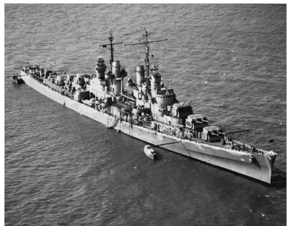
USS Atlanta (CL-51) on trials in 1942 showing seven of her eight 5"/38 (12.7 cm) Mark 29 twin mountings. Note the wing or broadside mounting, which was installed only on the first four ships of this class. U.S. Naval Historical Center Photograph # NH 57453. Photograph courtesy of Preston Cook.
