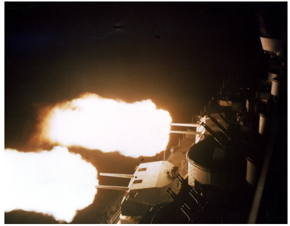
Twin 5"/38 (12.7 cm) Mark 28 mounts on USS Missouri (BB-63) in action during a night gunnery practice in August 1944. The Mark 28 mounting was used on all US Battleships completed during the 1940s. U.S. Naval Historical Center Photograph # 80-G-K-4550.
