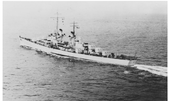
USS Atlanta (CL-51) on trials in 1942 showing seven of her eight 5"/38 (12.7 cm) Mark 29 twin mountings. Note the wing or broadside mounting, which was installed only on the first four ships of this class. U.S. Naval Historical Center Photograph # NH 57453. Photograph courtesy of Preston Cook.
