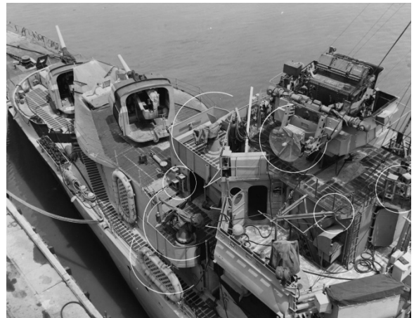
Bow of USS Mahan (DD-364) in June 1944. Another view of the Mark 21 open-back shield pedestal mounts. Note the groove in the deck of Mount #2. This was to allow a path for ejected cartridge cases when the gun was at high elevations. The later base ring mounts had the gun mounted a few inches higher and so did not need this groove. Note the Mark 33 director and its newly added radar and the non-slip tread material patterns on the decks. Also note the large "spray shield" around Mount 52. This shield was actually meant to protect the gun crew
