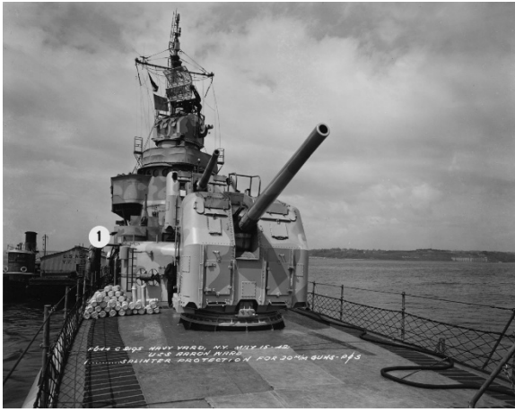
Mark 30 single mounts on USS Arron Ward (DD-483), a Gleaves class (DD-423) destroyer, in May 1942. Note 5" (12.7 cm) propellant canisters on the left and Mark 37 GFC director with Mark 4 "FD" Radar. U.S. Naval Historical Center Photograph # 19-N-30722.
