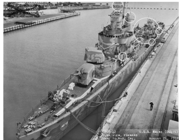
Mark 30 single mounts on USS Walke (DD-416) in August 1942. USS Walke was a Sims class (DD-409) destroyer, the first ships to have the Mark 37 GFCS (Gun Fire Control System), shown here having recently added a Mark 4 "FD" radar on top of the director. U.S. Naval Historical Center Photograph # 19-N-33273.
