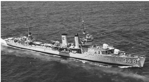
USS Farragut (DD-348) in April 1938. She was the first U.S. warship commissioned with 5"/38 (12.7 cm) Mark 12 guns. Note #3 gun directly behind the second funnel, the 0.50" BMGs directly in front of the bridge and that the funnels are closely spaced, indicating that she did not have unit machinery. U.S. Naval Historical Center Photograph # NH 80-G-465921, courtesy of NavSource .
