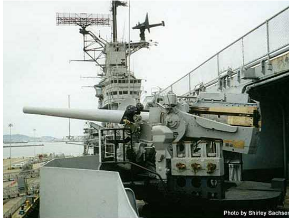
Figure 4 5"/38 (12.7 cm) Mark 24 pedestal mount on USS Hornet (CV-12). Note the fuze setting machine. Photograph copyrighted by Shirley Sachsen and used here by her kind permission.
