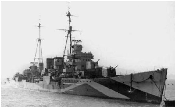
HMS Delhi after being refitted in the USA with five 5"/38 (12.7 cm) Mark 30 mounts and two Mark 37 GFCs. Note that the Mark 37 directors are equipped with British radars. Photograph courtesy of Steve Johnson of Cyberheritage .
