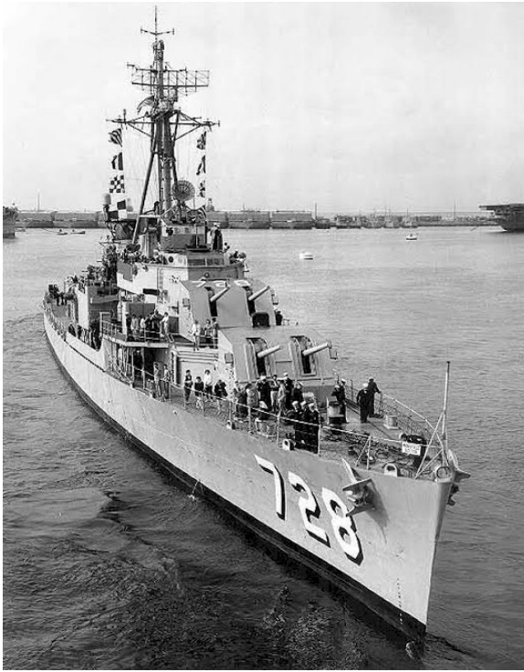
USS Mansfield (DD-728), an Allen M. Sumner class (DD-692) destroyer, in 1959 showing her bow Mark 38 mountings. Note the reinforcing added to Mount 51 to combat water damage. Photograph copyrighted by Richard Miller BMCS USNR RET.
